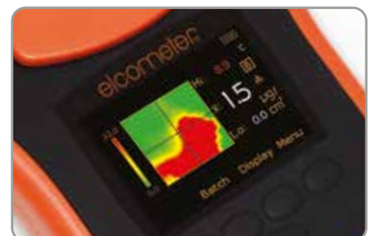
2D Salt Density Map with High/Low Readings
