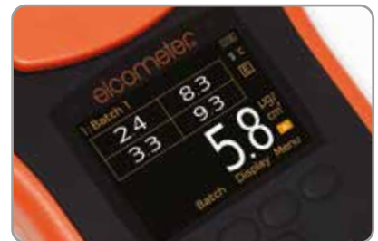
Four Bresle Patch Equivalent Readings
