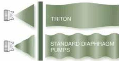
Triton pump provides 50% less pressure pulsation than standard diaphragm pumps.
