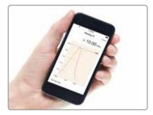
Using wireless Bluetooth<sup>®</sup> communication link the gauge to an Android<sup>™</sup> or iPhone<sup>‡</sup> mobile device. Live GPS coordinates from your mobile device can be added to reports and emailed instantly.
