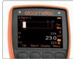
During a scan the live reading together with an analogue bar graph is displayed
