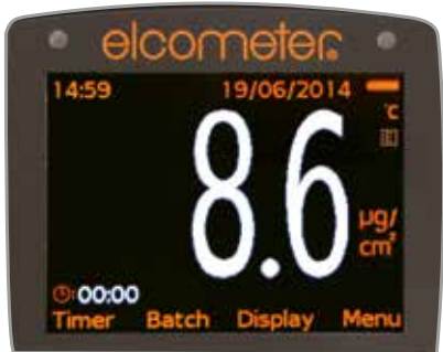
Large colour LCD screen displays readings in µg/cm², ppm, µS/cm, mS/cm, % salinity or mg/m²
