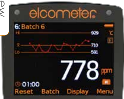
On-screen run graph shows last 20 measurement values
