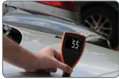
Measures on steel & aluminium body panels 2
