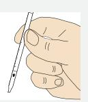
4. Insert sleeve with extract 5. Immediately remove solution and titration tube and read the number on into the hole previously the titration tube at the made in the box lid and interface of the colour change. Pink is normal, white is the chloride level.
